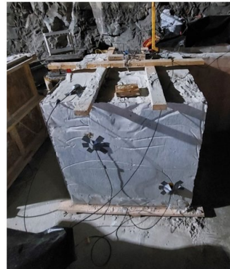
Figure Sensors installed on the sample of Mixture D.
