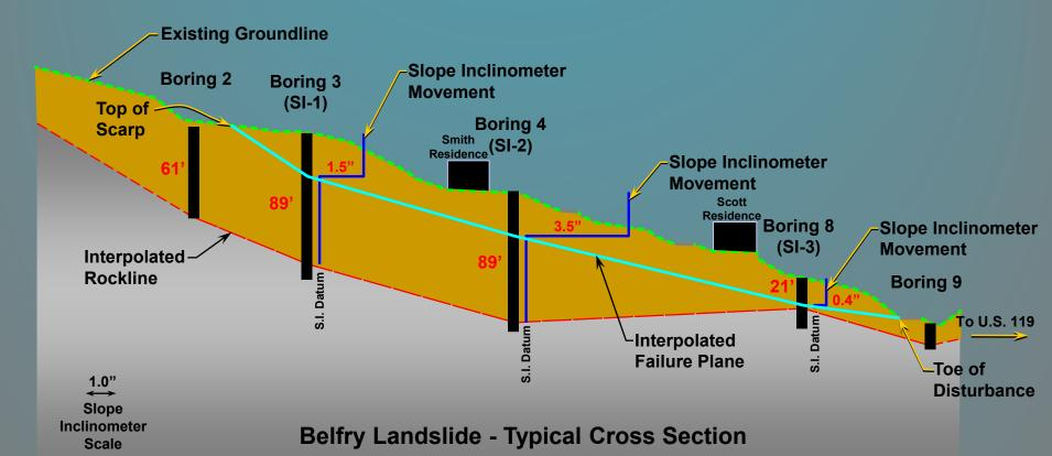
...to Determine Approximate Failure Plane Location and Calculate Residual Shear Strength of Colluvium
