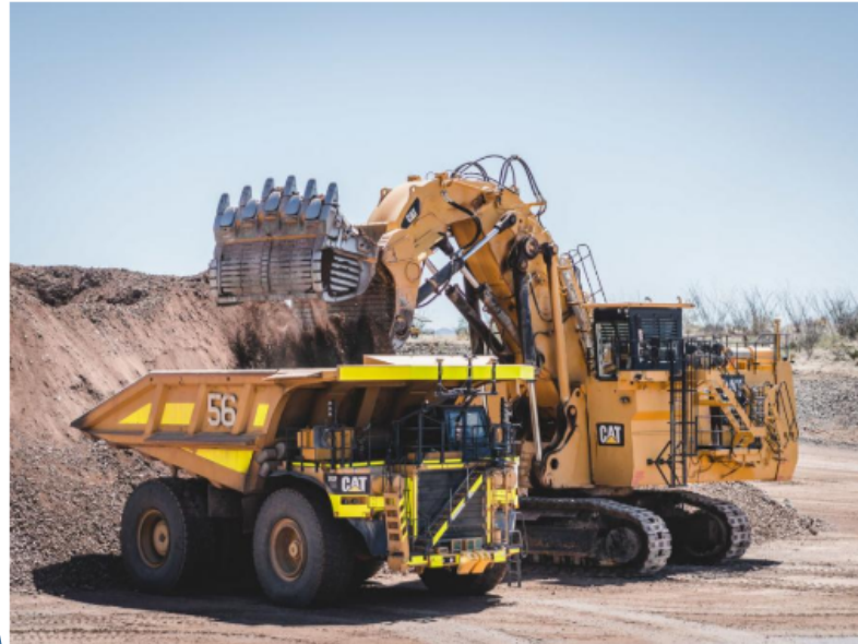
In the most remote places on earth, trucks hauling an upwards of 400 tons — about the weight of 200 cars — roam from pit to crusher with no humans in sight. These trucks are part of Caterpillar's Cat Command for Hauling system, commonly referred to as autonomous trucking. (Aaron Witt photo)
