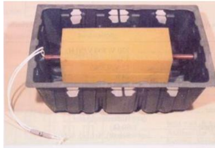
Water trough with built-in ignition system Water distribution of the barrier (DuPlessis and VanNiekerk, 2002)
