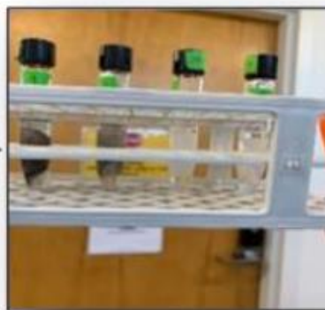
Filter transferred to the tube with Isopropanol
