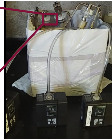
Laboratory sampling setup (respirable dust from source materials)
